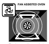
Top heat and bottom bake elements are used in conjunction with the fan.
